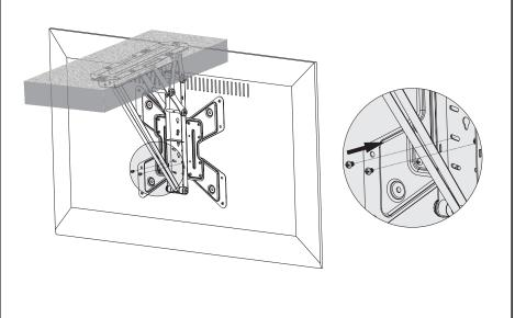
Clearance between the ceiling and top edge of TV should be no less than 15mm when TV is in the fully lowered position.
